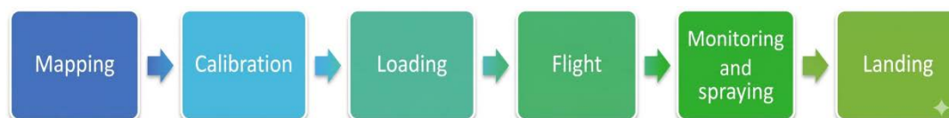
Figure 3. Flow chart of working of drone in pesticide application
