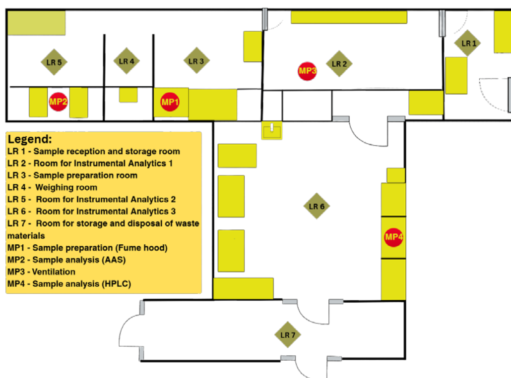
Figure 1. Measuring points of noise levels in laboratory for environmental and occupational monitoring
