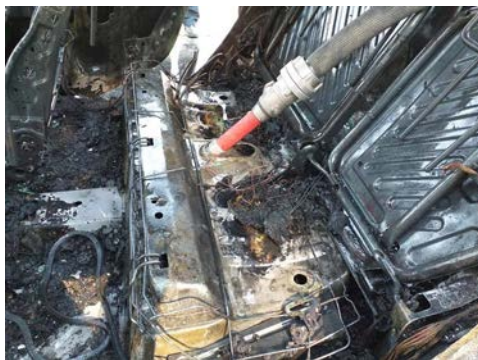
Figure 6. Extinguishing of high-voltage battery with fireman access mechanism
