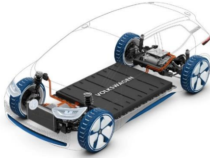
Figure 4. Battery location in the vehicle safety zone (Markus, 2016)
