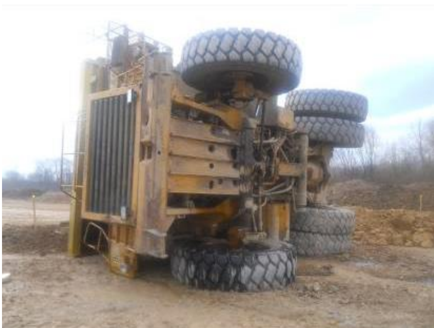
Figure 2. Photo of incident situation which consequences are overturn of dumper
