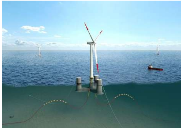
Figure 1. A Creative Commons licensed conceptualization for offshore floating wind turbine (Pegalajar-Jarudado, 2024).
