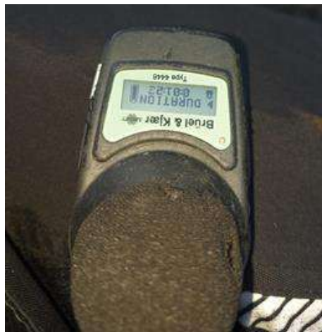
Figure 2. A personal noise dosimeter attached to the shoulder of the operator
