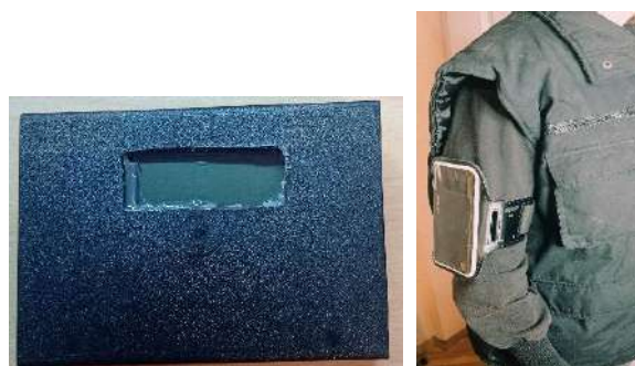
Figure 2. Photo of dosimeter in the box and in carrying position on the employee
