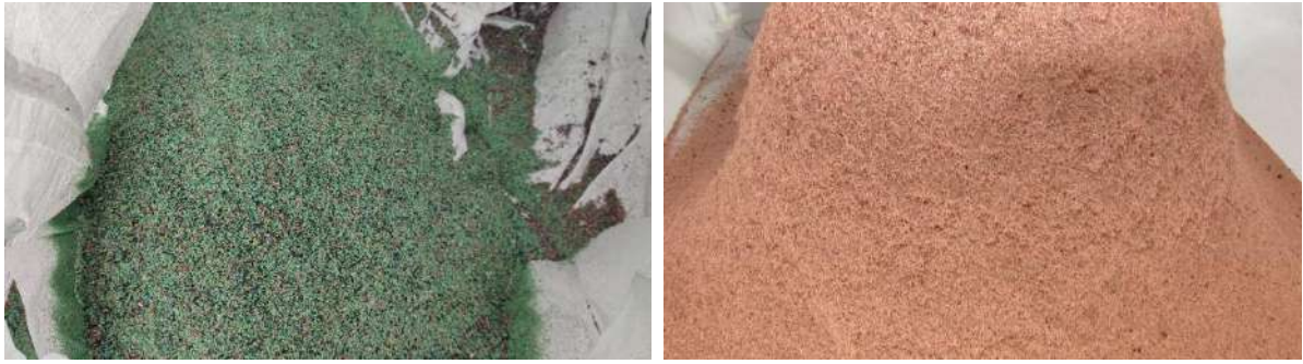
Figure 4. Plastic and copper granulate
