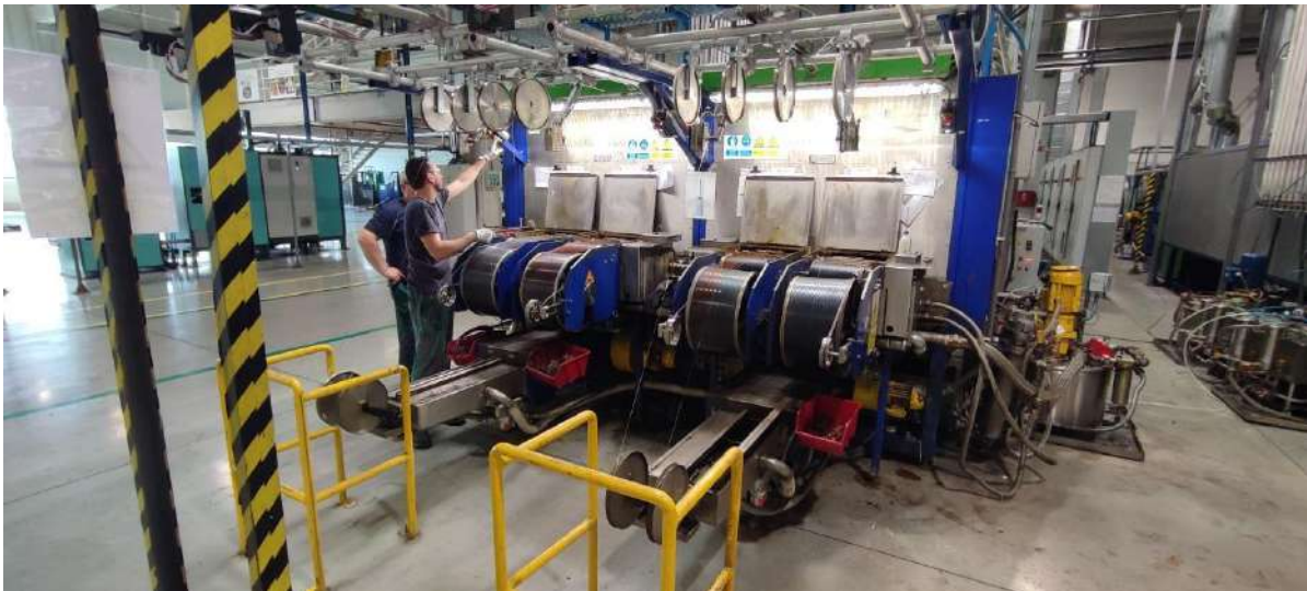
Figure 1. The process of applying enamel to copper wire
